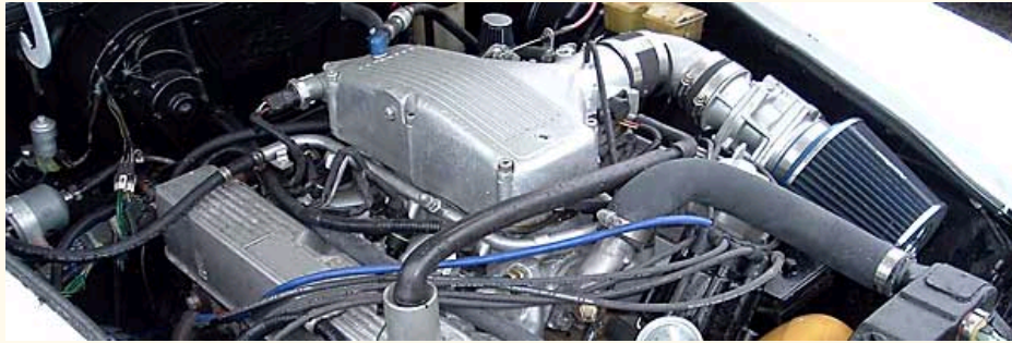
A Rover 14CUX Electronic Fuel Injection Installation (Installed by Glen Towery. Photo by Greg Myer.)
